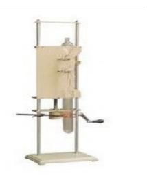
provided on the stand below the pipette. The depth of immersion is measured by a scale graduated in mm at the side of the sliding panel. Supplied complete with Anderson pipette 10 ml. at the side capacity made from glass, and a sedimentation tube also of glass of 500 ml capacity and 50 Nos Test forms.
